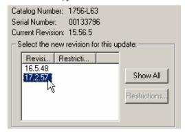
TIP If you are using a 1756-L7x controller and experience a Script File Error after selecting the firmware revision number (see the following example), there is likely an anomaly with your firmware files.
