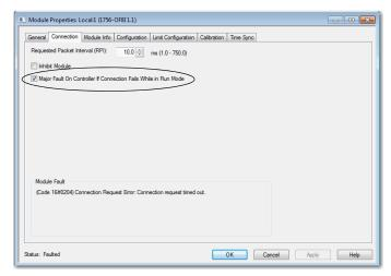
When you are monitoring the configuration properties of a module in the Logix Designer application and receive a Communication fault message, the Major Faults tab indicates the type of fault under Recent Faults.
