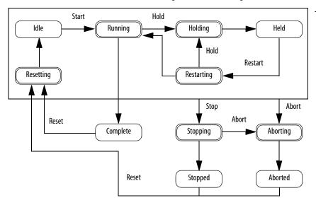
Your equipment can go from any state in the box to the stopping or aborting state.
