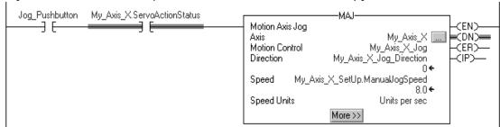
If Jog\_Pushbutton = off then the MAS instruction stops the axis at 100 units/.second<sup>2</sup>. Make sure that Change Decel is Yes. Otherwise, the axis decelerates at its maximum speed.
