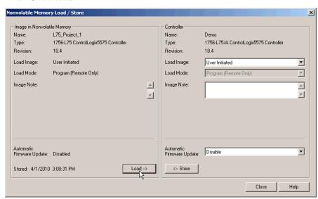
After clicking Load, the project is loaded to the controller as indicated by the controller status indicators.
