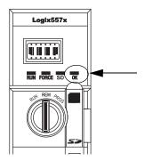
2. Leave the ESM on the controller until the OK status indicator is Off.
