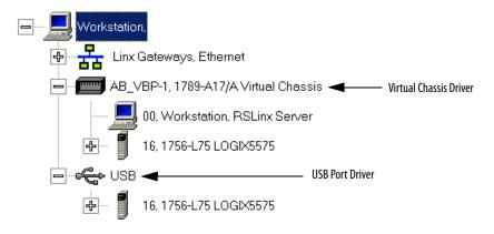
Your controller appears under two drivers, a virtual chassis and the USB port. You can use either driver to browse to your controller.
