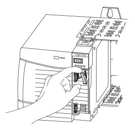
3. Press and release the SD card to eject it.
