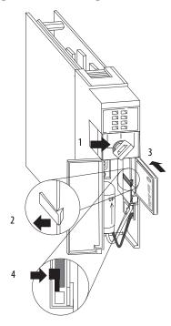
1. Open the door of the controller and push the CompactFlash latch to the left.
