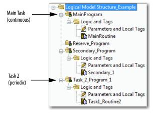
A task provides scheduling and priority information for a set of one or more programs. Configure tasks as continuous, periodic, or event by using the Task Properties dialog box.
