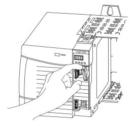
3. Insert the SD card into the SD card slot.
