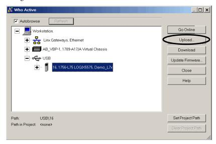
**2.** Click Upload after verifying the project that you are uploading in the Connected to Upload dialog box.
