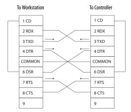
Plug the controller end of the serial cable into the RS-232 port on the front of the controller.
