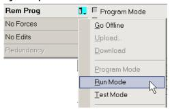
**TIP** For this example, the controller mode switch is set to Remote mode. If your controller mode switch is set to Run or Program modes, the menu options change.
