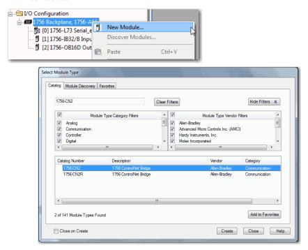
Specify the communication module properties according to your network configuration.
